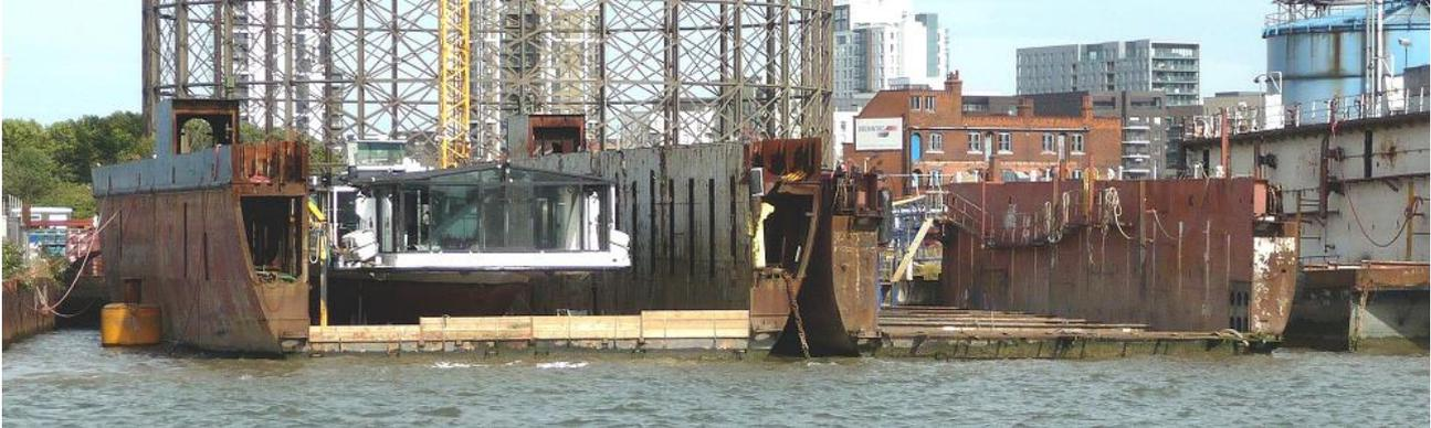
When the work is completed the cocks of the floating dock are opened and the dock sinks to the bottom again, the repaired vessel floats off. We are now ready for the next vessel. The procedure above has been completed without recourse to energy-expensive pumping.
