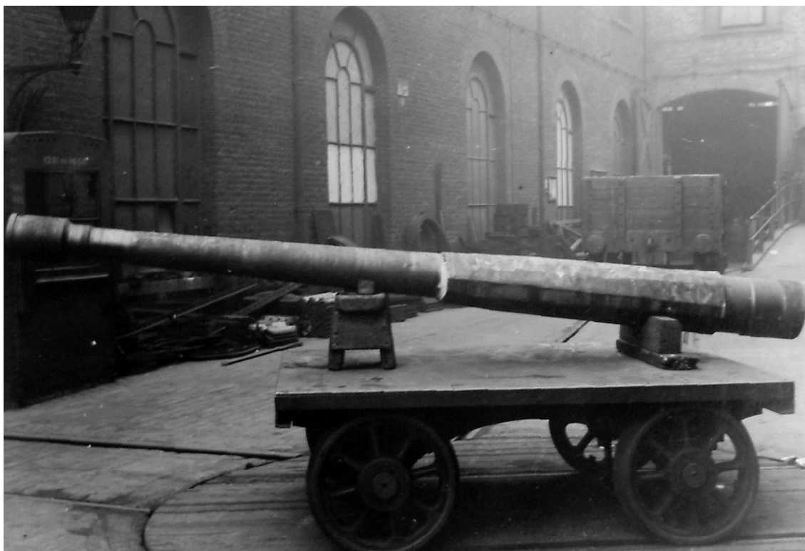
Figure 9. Jacket for Quick-Firing (QF) 3" gun on turntable at Stratford Locomotive Works, circa 1915–18
